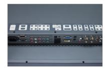
Mutiple video inputs (VGA, DVI, dual BNC, S-Video and Component) allow for effortless system integration
