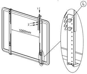
12. HANG BOARD ON FRAME Make projector level and turn on. Set projector zoom as large as possible. Adjust boom length so image is same size as board. Hang board at same height as image.
