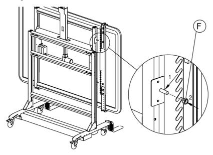
13. TEST EXCURSION Plug motor into power and move assembly to upper and lower limits to ensure no snags and mount is operating safely.
