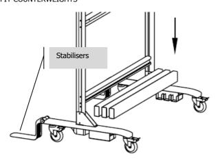
NOTE: Stabilisers should only be raised to move product. To unlock squeeze hinge.
