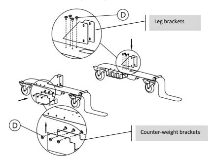
2. ASSEMBLE LEGS Ensure rails are correct way up as shown.
