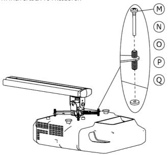
10. FIT PROJECTOR ASSEMBLY TO BOOM Tighten screw to lock the two parts of the boom together
