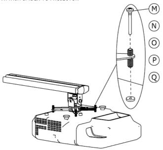
7. FIT PROJECTOR ASSEMBLY TO BOOM Tighten screw to lock the two parts of the boom together
