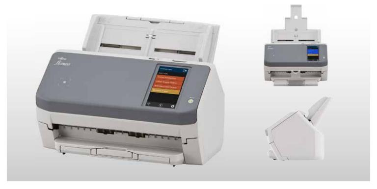
Based on the world's most trusted scanning technology, the fi-7300NX delivers flexible, centralised capture for organisations with distributed teams or scanning needs. It can hold up to 80 sheets at a time, scanning 300 dpi A4 portrait at 60 ppm (120 ipm duplex).
