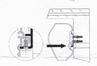
Afterwards tighten the securing screw, Prevention the screw comes out from wall mount bracket.
