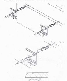
Mark 2 horizontal parallel lines on wall at desired height. Drill holes on wall According to the openings on wall mount bracket
