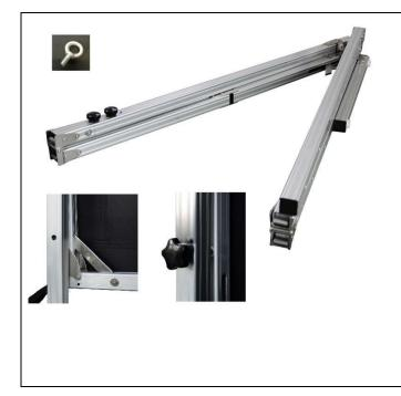
The FP series frame is based upon the latest click-frame system for a strong and durable frame which is easily assembled. The 3.2cm tube alloy frame also comes with sturdy, removable legs. If legs are not required the screen may be suspended using ring-bolts attached to fly-points in the frame. Without the legs the FP series may be suspended either in landscape or portrait via fly points (ringbolts) built into the frame.
