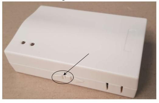
2. Press the program setting button on the back of the handheld remote with a Pen until the LED on the wired controller stops flashing
